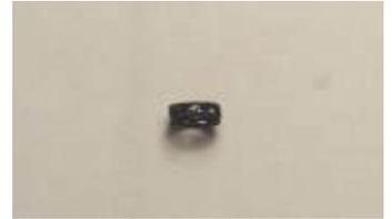
If heavy side pressure on the handpiece is used it will cause the bearing balls to roll vertically in the retainer. The holes will enlarge causing increased radial play of the bur.
